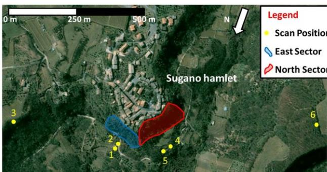
Fig. 2 – Identification of scan positions on satellite image.
