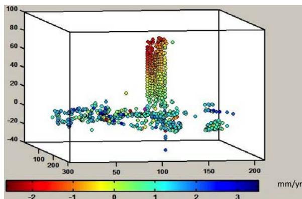
Figure 4. PS related to a high-rise building with a clear gradient of displacement along the structure.
