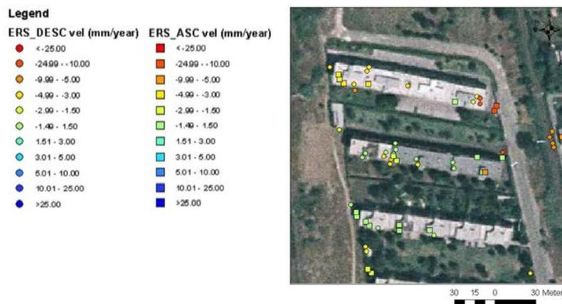
Figure 4. – Ascending and descending PS related to a couple of buildings (higher part of the picture) affected by differential settlement process (period: 1992-2001).
