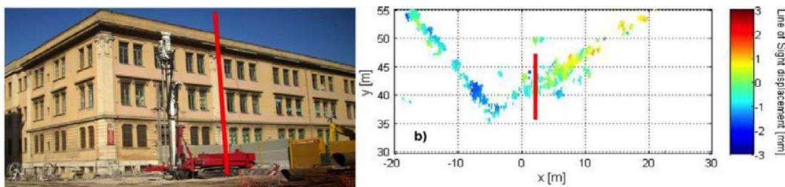
Figure 5. Picture of the building and displacements map derived by TInSAR. The red line identifies the same sector.
