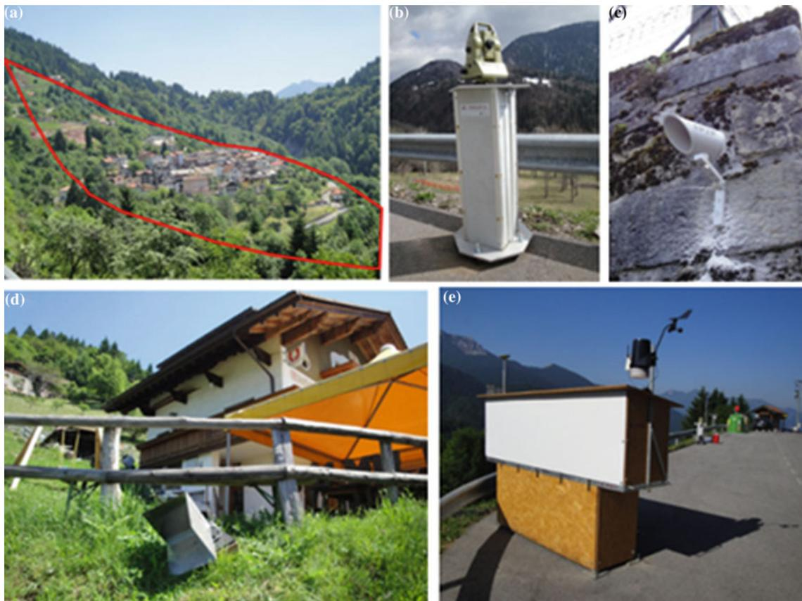
**Fig. 34.3** a Ligosullo landslide; b topographic monitoring platform; c topographic target; d TInSAR corner reflector; e TInSAR monitoring platform
