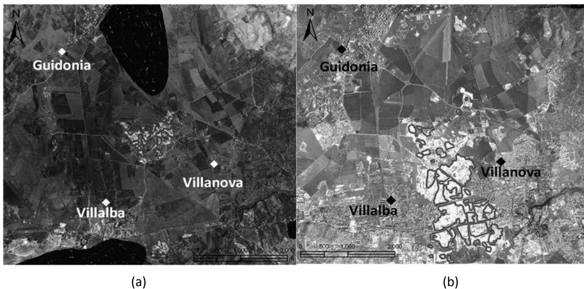
Figure 2 Evolution of the quarries activities in the plain: (a) the orthophoto represents the plain in 1954: the perimeter of each pit is shown by polygons; some obscured areas are depicted such as the Guidonia airport to the north, as required by the military regulations at the time; (b) the orthophoto represents the plain in 2005: the perimeter of each pit is shown by polygons. It is clear the huge expansion of the quarries area (modified from Floris et al. 2014)
