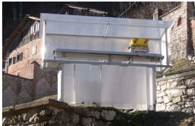
Figure 1. Picture of the TInSAR system IBIS-L by IDS S.p.A. installed on a QUIB basement by NHAZCA S.r.l.
